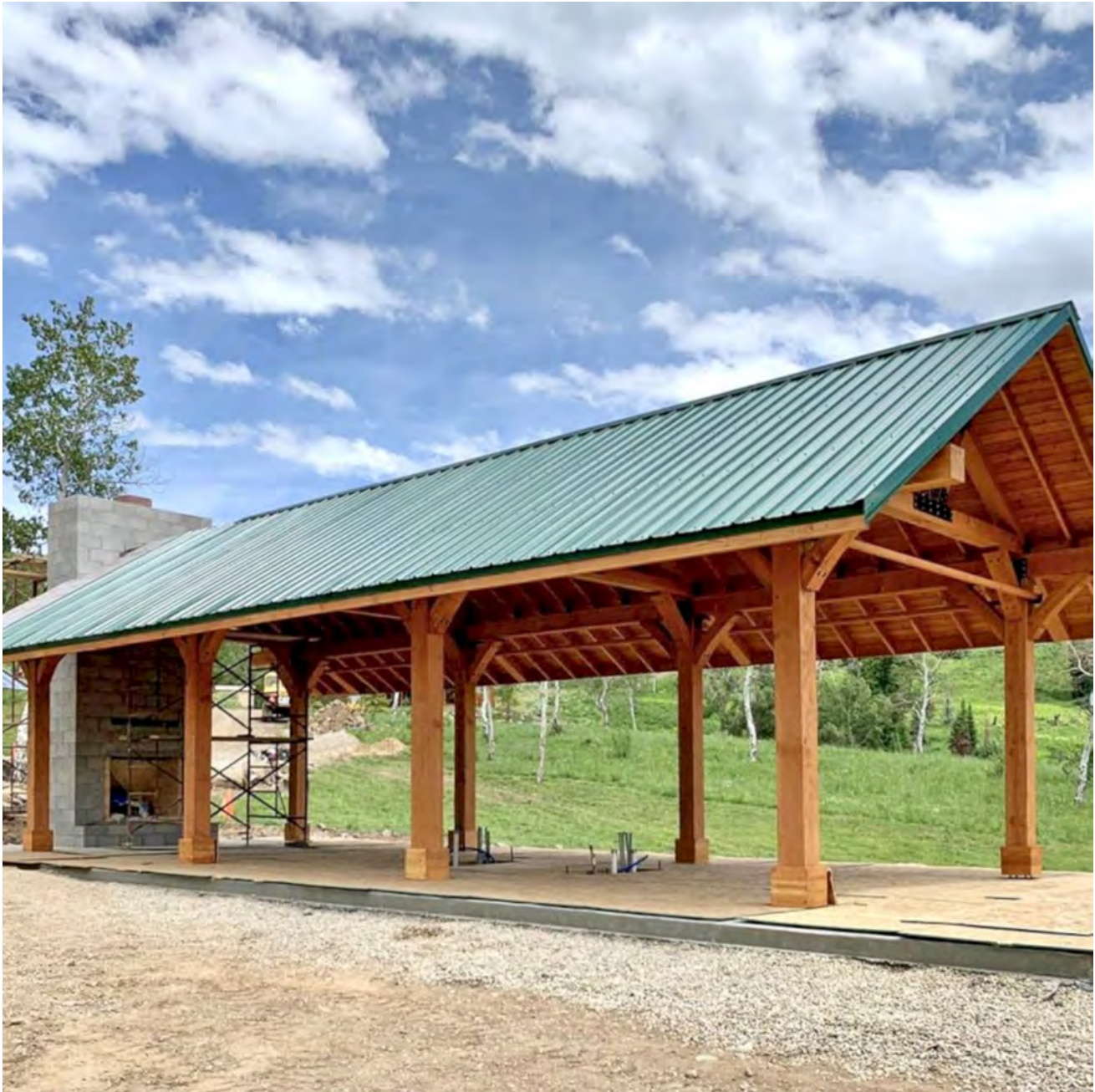
The Thick Timber Toledo Wood Pavilion (Options: 50' L x 24' W, Douglas-fir, 8-Post Anchor Kit for Gale-Wind, with Curtain Rods, Electrical Wiring Trim for 4 Posts, 10 x 10 Supports and Posts, 8 x 8 Rafters, Transparent Premium Sealant). Custom 4' Overhang on All Sides (Standard Overhang is 1'). Photo Courtesy of R. Barry of Hayden, Colorado.
