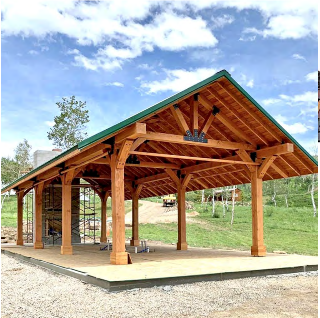
The Thick Timber Toledo Wood Pavilion (Options: 50' L x 24' W, Douglas-fir, 8-Post Anchor Kit for Gale-Wind, with Curtain Rods, Electrical Wiring Trim for 4 Posts, 10 x 10 Supports and Posts, 2 x 8 Rafters, Transparent Premium Sealant). Custom 4' Overhang on All Sides (Standard Overhang is 1'). Photo Courtesy of R. Barry of Hayden, Colorado.
