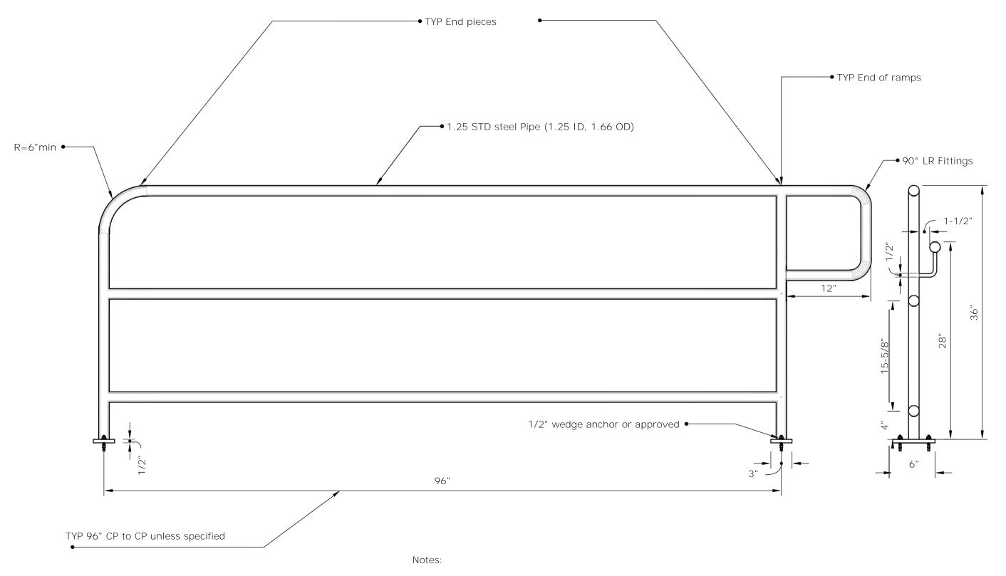
All vertical and horizontal members to be constructed using 1.25" STD steel pipe (1.25" I.D., 1.66" O.D.).TYP Finish Specification: Standard finish is powder coating.
